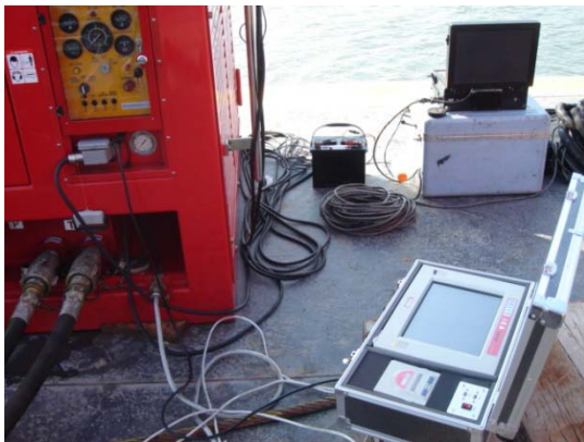
IEA is connected with hammer and power pack
