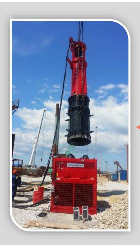
Hammer Capacity : 42 ton.m (412 kJ)
